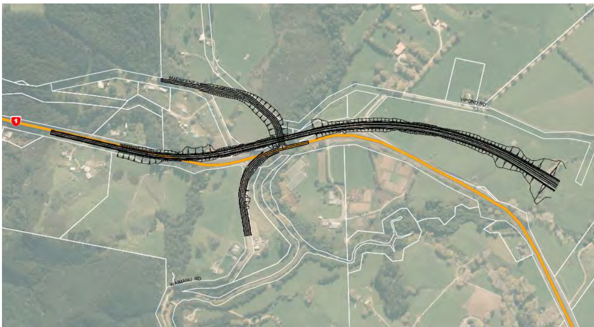
Figure 7-8: New offline bridge and grade separated intersection (JG02)
